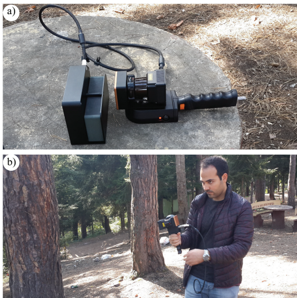
Figure 3. (a) General view of the Zeb-Revo instrument; (b) View of the instrument during data acquisition on plot 4 (Çscd2 stand).
